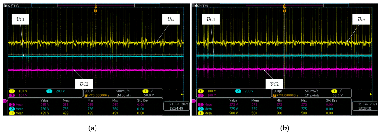
Figure 11. Waveforms of the input voltage, voltage across the capacitor C_1 , and voltage across the capacitor C_2 : the zero-sync method (a) and the conventional method (b).
