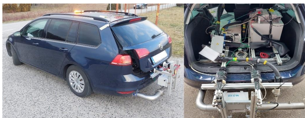
Figure 1. Test vehicle with built-in measuring equipment.
