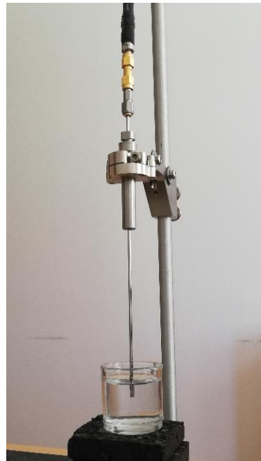
Figure 1. The slim form inserted into a liquid MUT.
