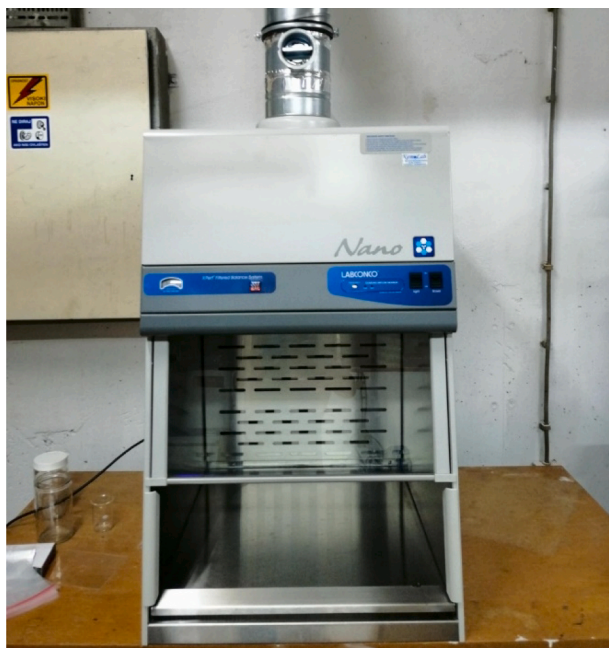
Fig. 1. LABCONCO XPert Nano Enclosure powder weighing station.
