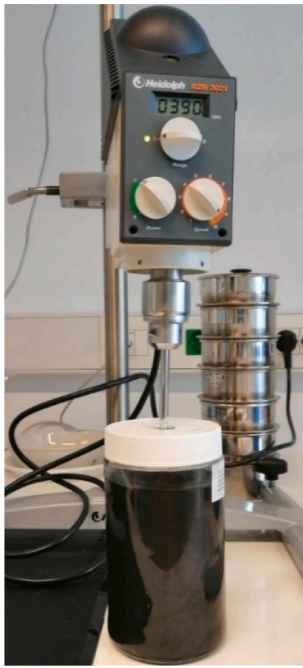
Fig. 5. Mechanical stirring of NEPCM.
