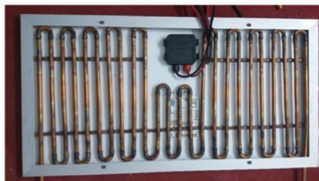
Fig. 9. PVT-PCM solar collector [37].
