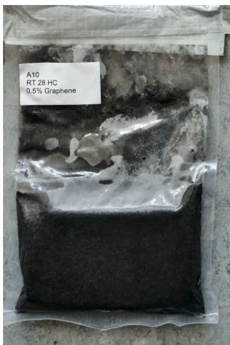
Fig. 2. Example of Graphene/RT28 HC sample in two-layer PA/PE bags.
