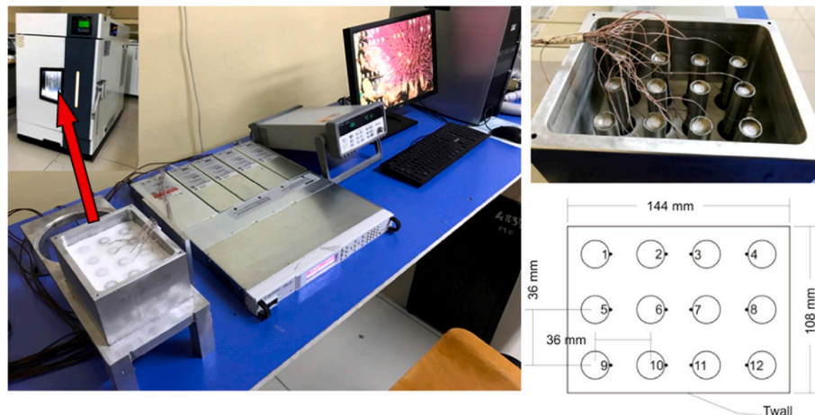
Fig. 12. Experimental layout of the simulated battery pack, [43].
