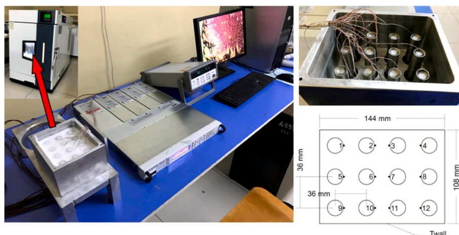
Fig. 12. Experimental layout of the simulated battery pack, [43].
