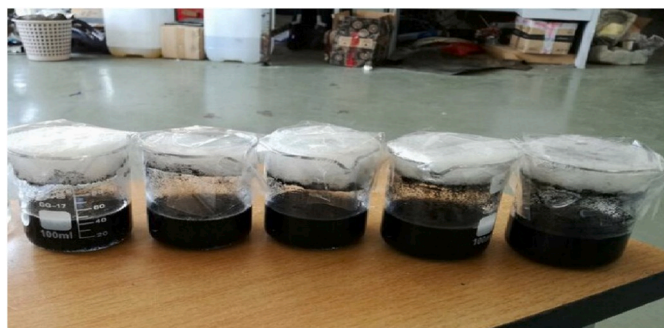
Fig. 17. Multi-walled carbon nanotubes (MWCNT) nanofluids, [52].
