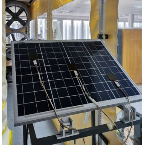
Figure 8.1. Experimental test rig layout in wind tunnel [117].
