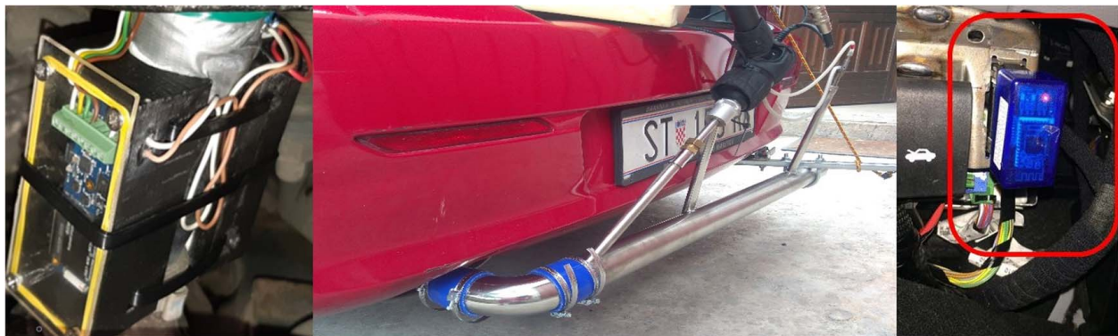
Fig. 2 Measuring equipment installed on the vehicle: Torque and power measurement device, gas analyzer, Pitot connection, and OBD connection
