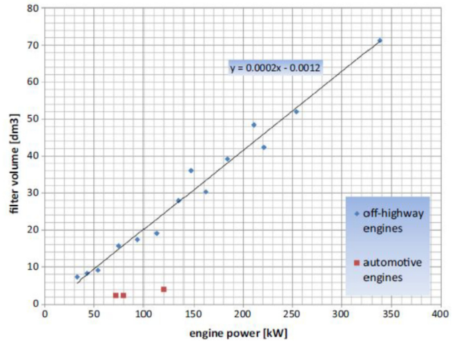
Fig. 27. vol ratio of DPF filters to maximum engine power, Stamatellou et al. (2017).
