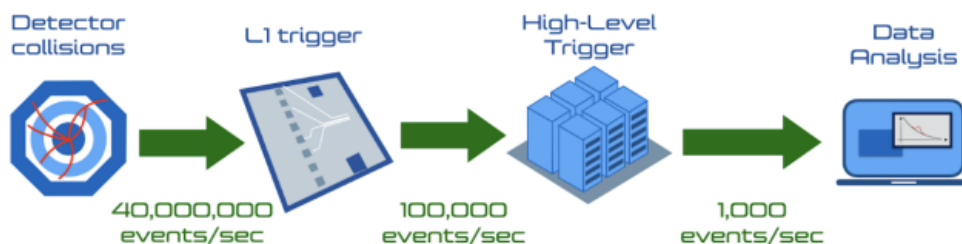
Figure 2.5. The data processing flow in CMS experiment: Forty million collisions are generated per second. The L1T selects 100 000 events, which are then passed to HLT. Only 1000 events per second are kept for further studies [48].
