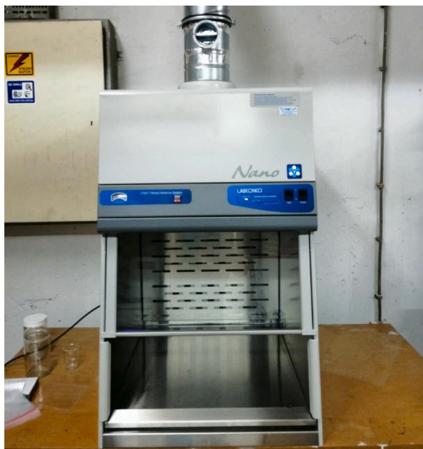
Fig. 1. LABCONCO XPert Nano Enclosure powder weighing station.
