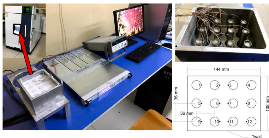
Fig. 12. Experimental layout of the simulated battery pack, [43].
