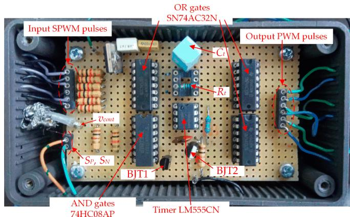
**Figure 7.** Photo of the electrical circuitry utilized for the STSs injection.
