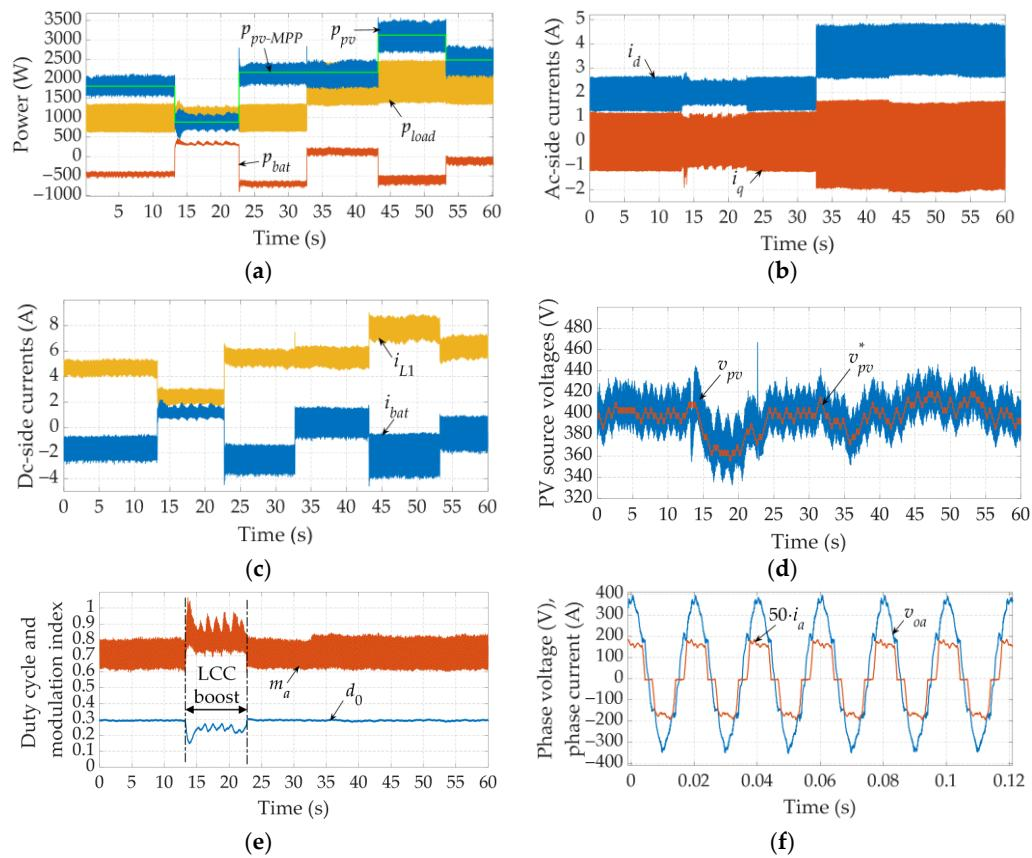
**Figure 20.** Irradiance variation and non-linear load resistance variation during the stand-alone operation: system powers (a), output load currents (b), dc-side currents (c), PV source voltage (d), modulation index and duty cycle (e), and phase voltage and current (f).
