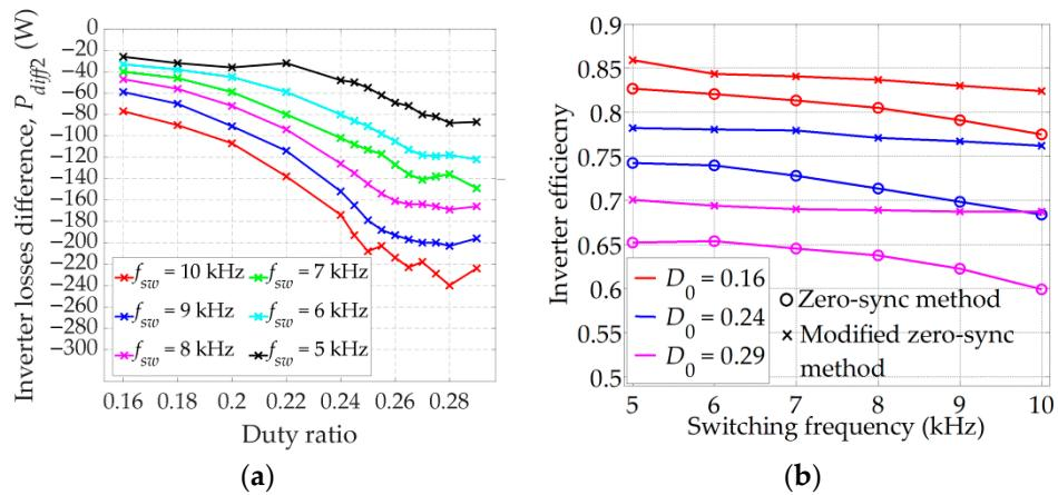
**Figure 20.** Inverter losses difference ( $P_{diff2}$ ) as a function of the duty ratio for different switching frequencies (a); inverter efficiency as a function of the switching frequency for different duty ratio values (b).
