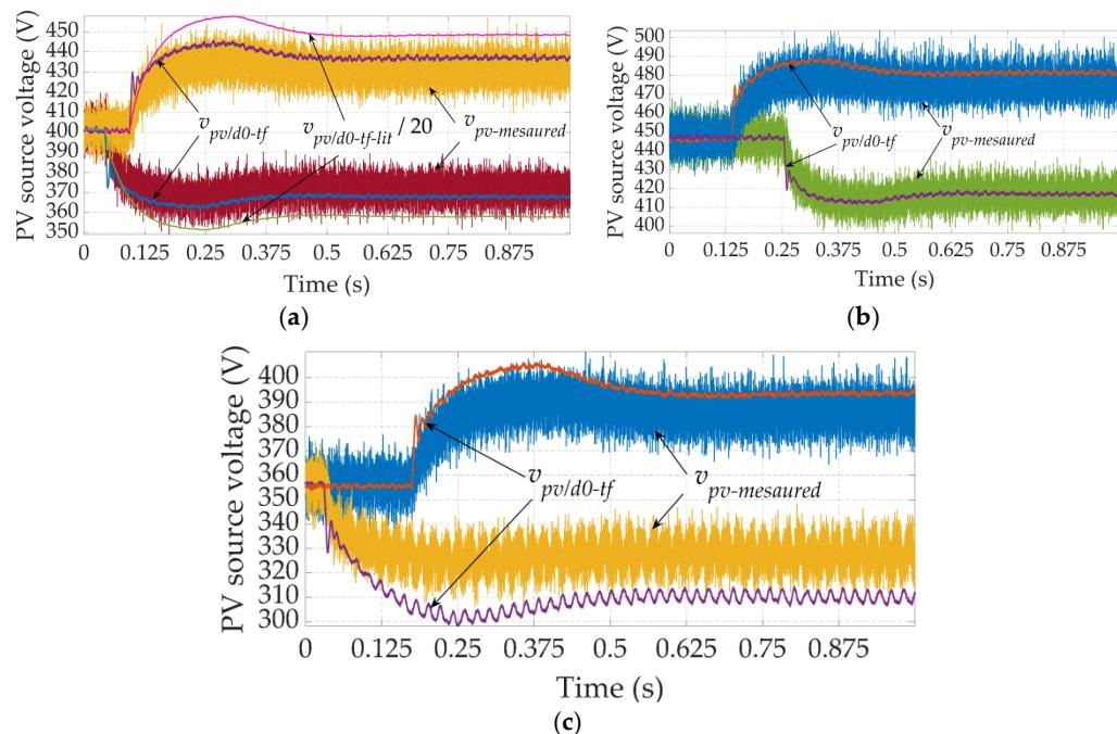
**Figure 11.** Waveforms of the PV voltage obtained by the transfer function and by measurement during transients for:  $Z = 600 \text{ W/m}^2$ ,  $T_{pv} = 30^\circ\text{C}$  (linearization point) (a),  $Z = 600 \text{ W/m}^2$ ,  $T_{pv} = 10^\circ\text{C}$  (b), and  $Z = 600 \text{ W/m}^2$ ,  $T_{pv} = 50^\circ\text{C}$  (c).
