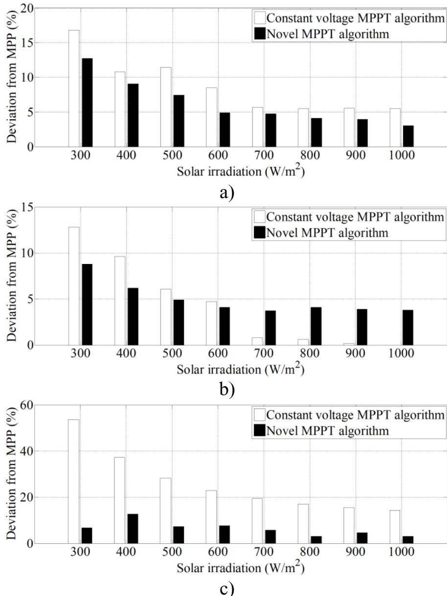
**Fig. 11.** Deviation from the MPP vs. solar irradiation level for the proposed MPPT algorithm and constant-voltage algorithm: a)  $T = 25^\circ\text{C}$ , b)  $T = 50^\circ\text{C}$ , c)  $T = 75^\circ\text{C}$ .
