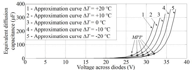
Fig. 12. Equivalent diffusion capacitance vs. voltage across diodes for different temperatures and constant nominal solar irradiation level
