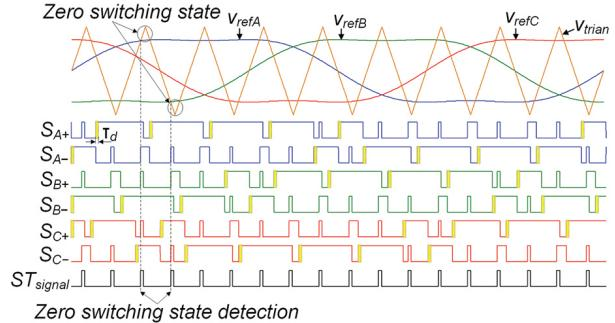
**Fig. 2.** Waveforms of the dead-time zero-sync SPWM [7]
