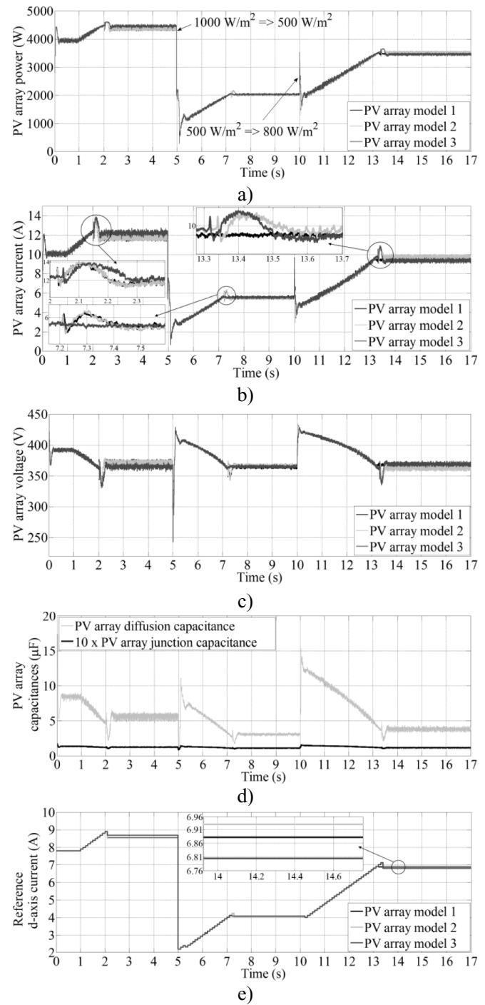
Fig. 9. Variables of the PV array for different solar irradiation levels and the constant PV array temperature ( $75^\circ\text{C}$ ): (a) power, (b) current, (c) voltage, (d) capacitances, (e) reference d-axis current.
