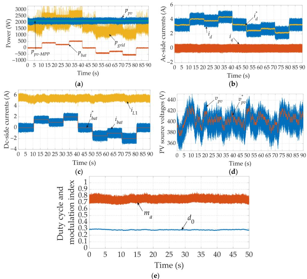
**Figure 18.** Reference battery current variation during the grid-tied operation: system powers (a), output grid currents (b), dc-side currents (c), PV source voltage (d), and modulation index and duty cycle (e).
