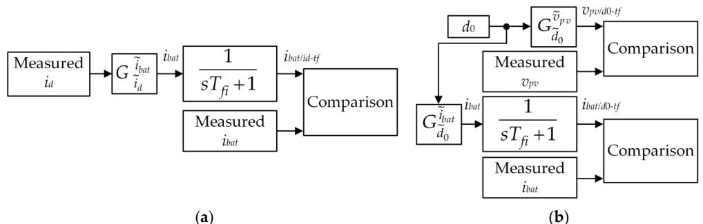
**Figure 9.** Setups utilized for the accuracy verification of transfer functions: from  $d$ -axis grid current to battery current (a), and from duty cycle to battery current/ PV source voltage (b).
