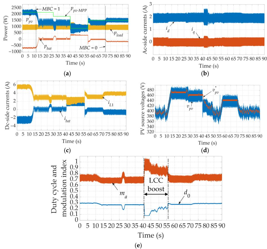
**Figure 21.** Irradiance variation and maximum battery charge signal variation during the stand-alone operation: system powers (a), output load currents (b), dc-side currents (c), PV source voltage (d), and modulation index and duty cycle (e).
