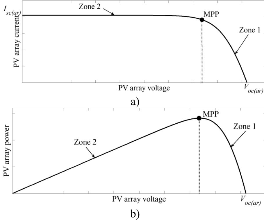
**Fig. 5.** (a) PV array static I-V characteristic, (b) PV array static P-V characteristic.
