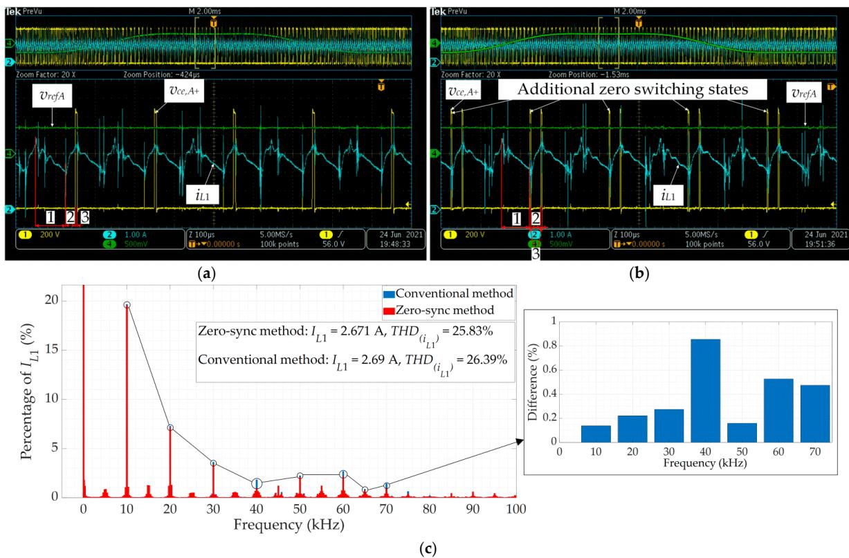
**Figure 10.** Waveforms of the reference voltage of phase A, collector-emitter voltage of the upper transistor in the phase A, and qZSI input current in case of implementing the zero-sync method (a) and the conventional method (b), the harmonic spectrum of the qZSI input current waveform (c).
