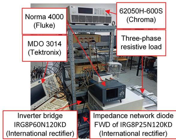
**Fig. 5.** Laboratory setup of the stand-alone qZSI-based system
