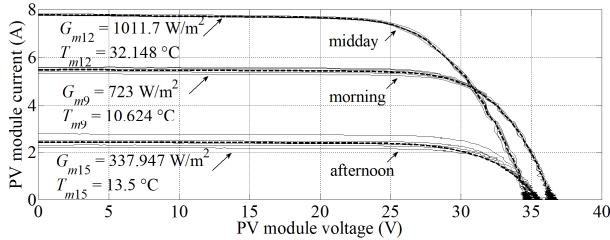
Fig. 4. The PV module experimental static I-V characteristics
