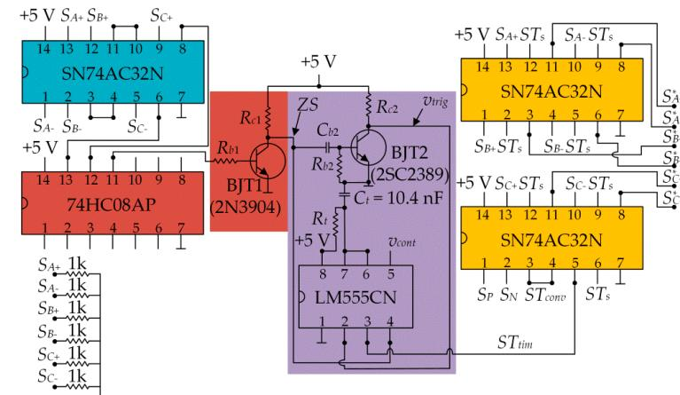
**Figure 5.** Electrical diagram of the PWM pulses generation with the STSs injection by means of both the zero-sync and conventional methods.
