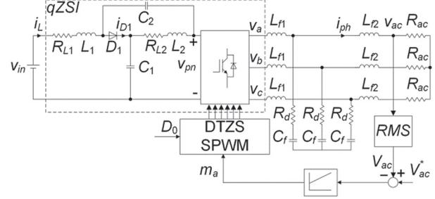
**Fig. 1.** Stand-alone qZSI-based control system [15]
