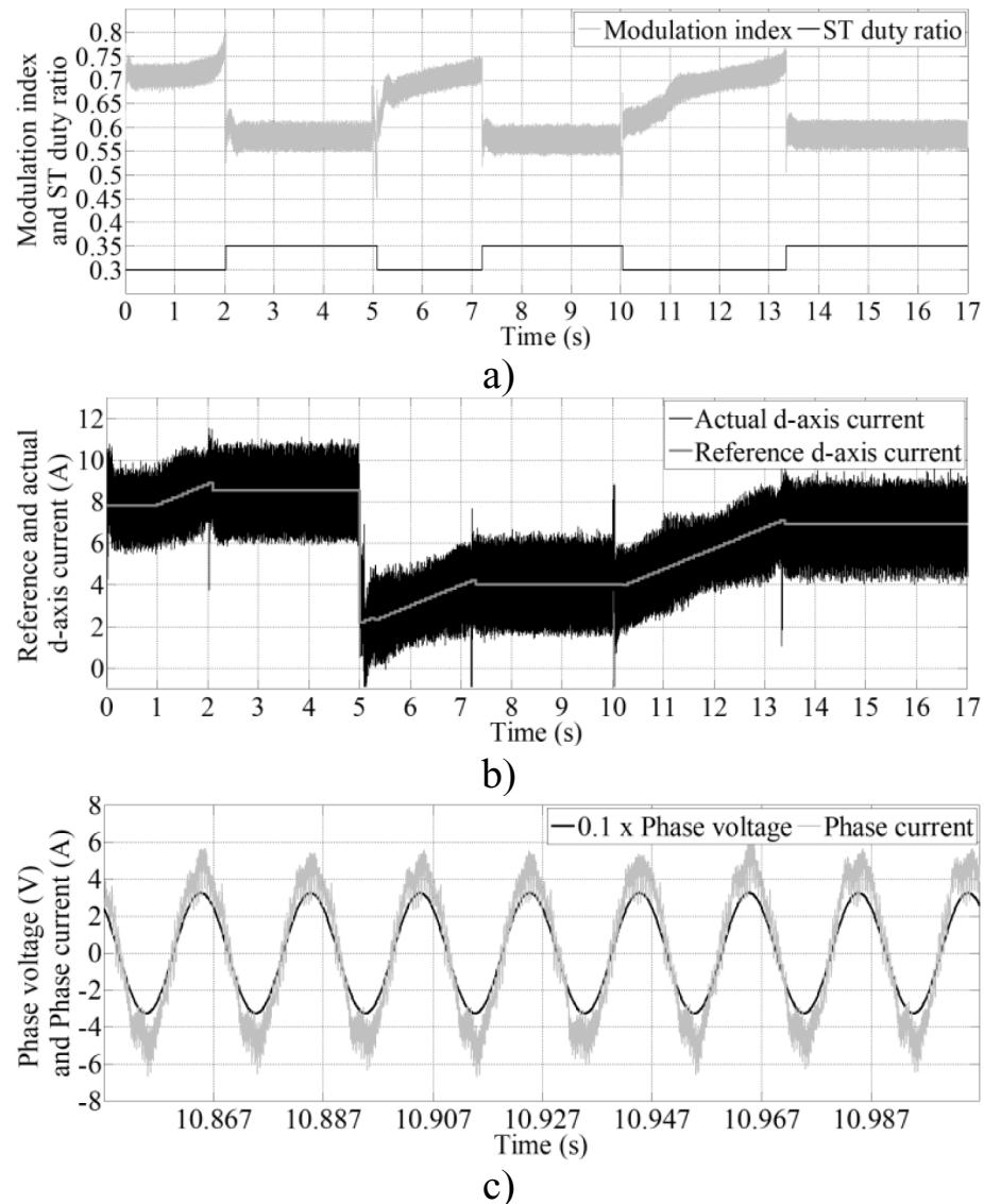
**Fig. 10.** Characteristic variables of the qZSI for different solar irradiation levels and the constant PV array temperature: (a) Modulation index, ST duty ratio, (b) Reference and actual d-axis current, (c) Phase current and voltage.
