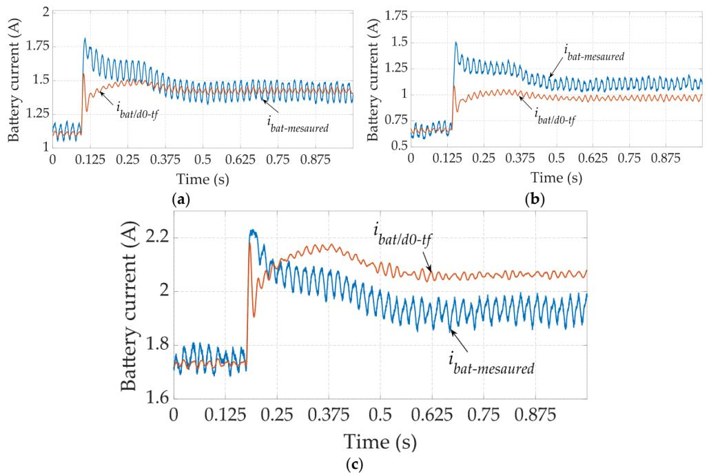
**Figure 12.** Waveforms of the battery current obtained by the transfer function and by measurement during transients for:  $Z = 600 \text{ W/m}^2$ ,  $T_{pv} = 30^\circ\text{C}$  (linearization point) (a),  $Z = 600 \text{ W/m}^2$ ,  $T_{pv} = 10^\circ\text{C}$  (b), and  $Z = 600 \text{ W/m}^2$ ,  $T_{pv} = 50^\circ\text{C}$  (c).
