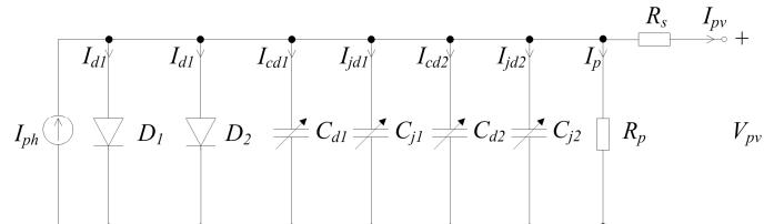
Fig. 6. Equivalent circuit of the proposed model of the PV module
