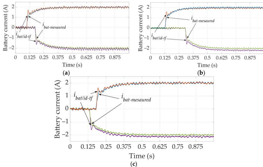
**Figure 10.** Waveforms of the battery current obtained by the transfer function and by measurement during transients for:  $Z = 600 \text{ W/m}^2$ ,  $T_{pv} = 30^\circ\text{C}$  (linearization point) (a),  $Z = 1000 \text{ W/m}^2$ ,  $T_{pv} = 10^\circ\text{C}$  (b), and  $Z = 500 \text{ W/m}^2$ ,  $T_{pv} = 50^\circ\text{C}$  (c).
