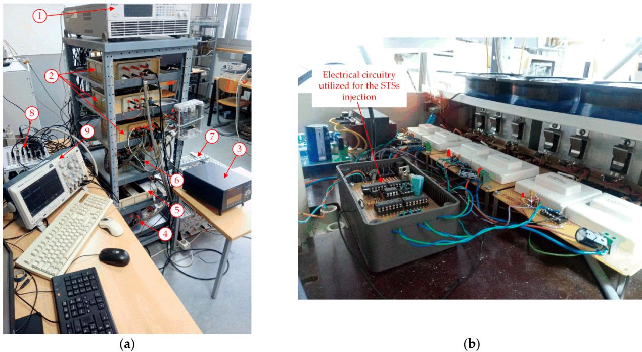
**Figure 8.** Laboratory setup of the qZSI in the stand-alone configuration (a), the qZSI three-phase inverter bridge (b).
