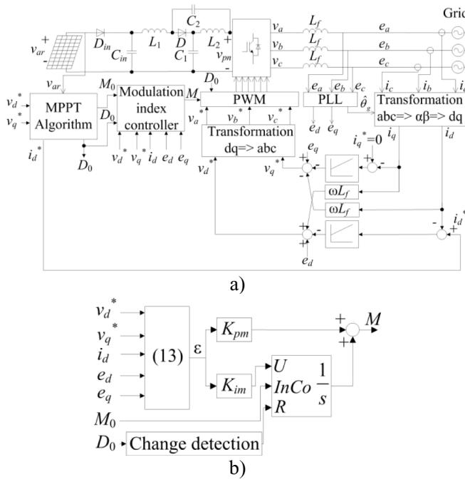
Fig. 4. (a) Structure of the proposed PV-qZSI control system, (b) modulation index PI controller.
