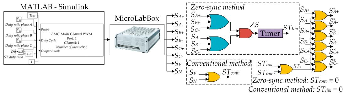
**Figure 4.** Logic diagram of the PWM pulses generation with the STSs injection by means of both the zero-sync and conventional methods.
