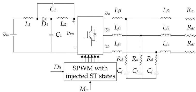
**Figure 1.** qZSI in a stand-alone configuration.
