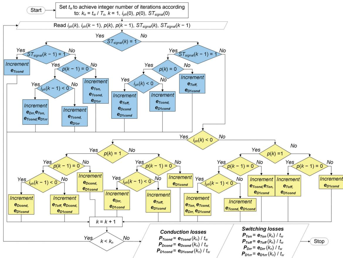
**Fig. 3.** Flow chart of the LCA [15]
