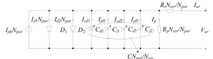
**Fig. 3.** Equivalent circuit of the variable-capacitance model of the PV array.
