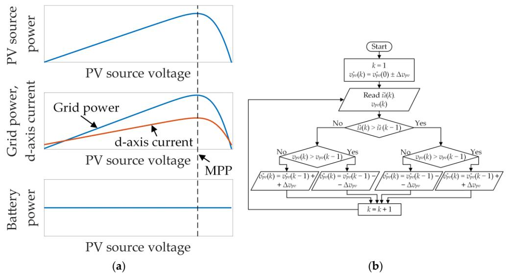
**Figure 6.** Grid-tied operation: PV source power, grid power and  $d$ -axis current, and battery power (a), and flow chart of the MPPT algorithm (b).
