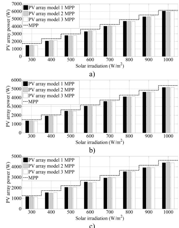
Fig. 7. PV array power vs. solar irradiation, for the different models of the PV array, and the PV array temperatures: (a)  $T = 25 \text{ }^{\circ}\text{C}$ , (b)  $T = 50 \text{ }^{\circ}\text{C}$ , (c)  $T = 75 \text{ }^{\circ}\text{C}$ .
