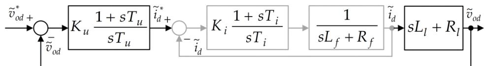
**Figure 4.** Control loop of the  $d$ -axis load voltage.
