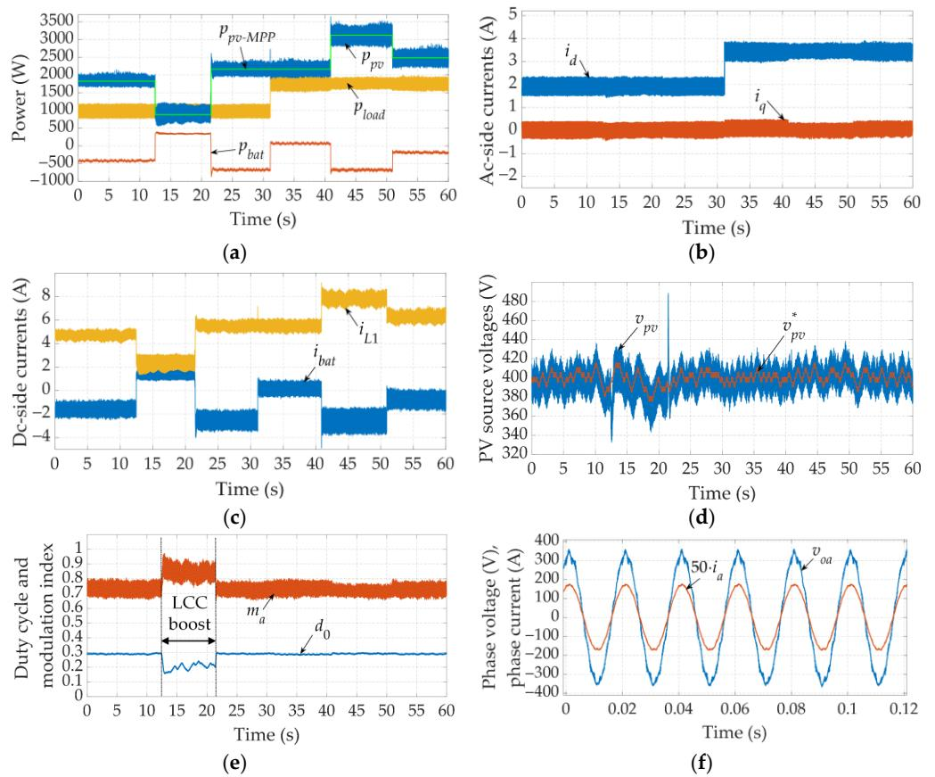
**Figure 19.** Irradiance variation and load resistance variation during the stand-alone operation: system powers (a), output load currents (b), dc-side currents (c), PV source voltage (d), modulation index and duty cycle (e), and phase voltage and current (f).
