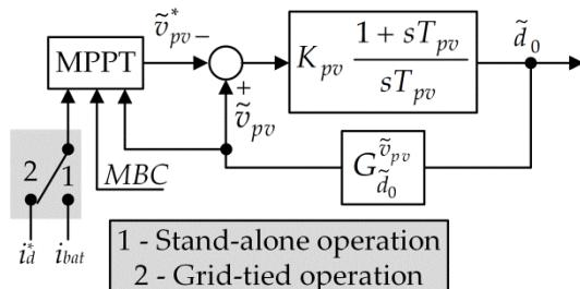
**Figure 5.** Control loop of the PV source voltage.
