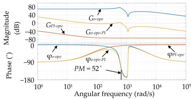
**Figure 15.** Bode plot of the PV source voltage control loop.
