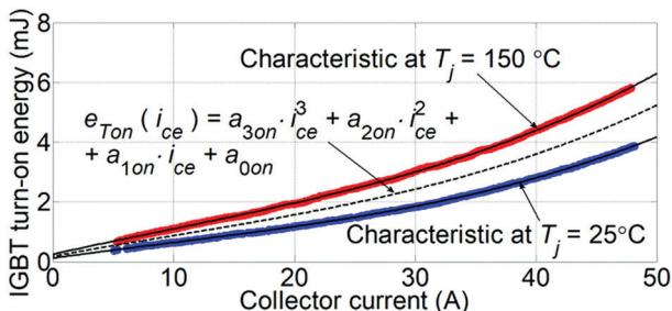
**Fig. 4.** Turn-on characteristics of the utilized IGBT [15]
