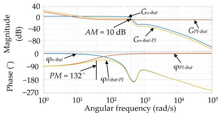
**Figure 13.** Bode plot of the battery control loop.
