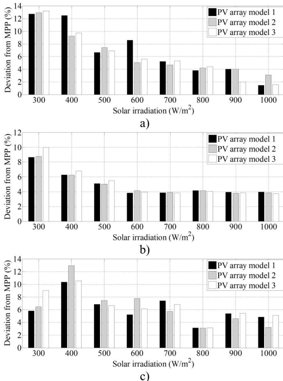
Fig. 8. Deviation from MPP vs. solar irradiation for the different models of the PV array, and the PV array temperatures: a)  $T = 25^\circ\text{C}$ , b)  $T = 50^\circ\text{C}$ , c)  $T = 75^\circ\text{C}$ .
