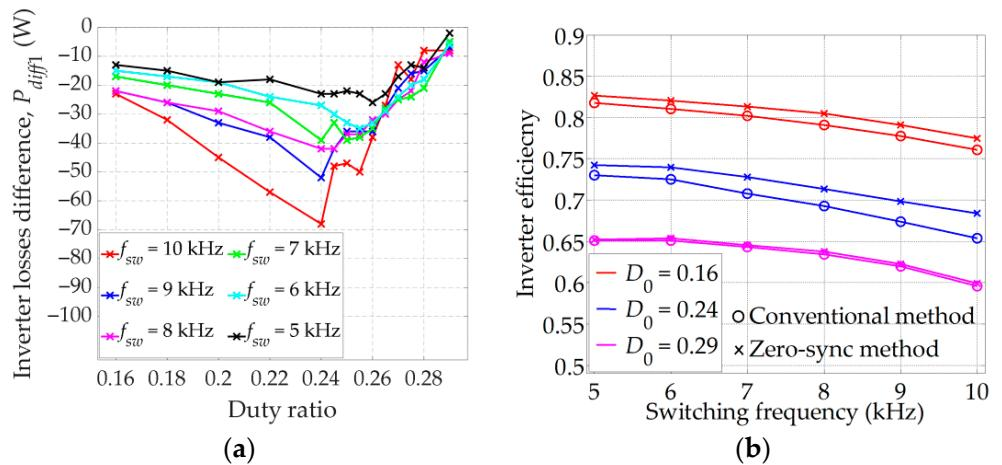
**Figure 14.** Inverter losses difference ( $P_{diff1}$ ) as a function of the duty ratio for different switching frequencies (a); inverter efficiency as a function of the switching frequency for different duty ratio values (b).
