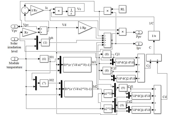
Fig. 7. Proposed PV model in MATLAB-Simulink
