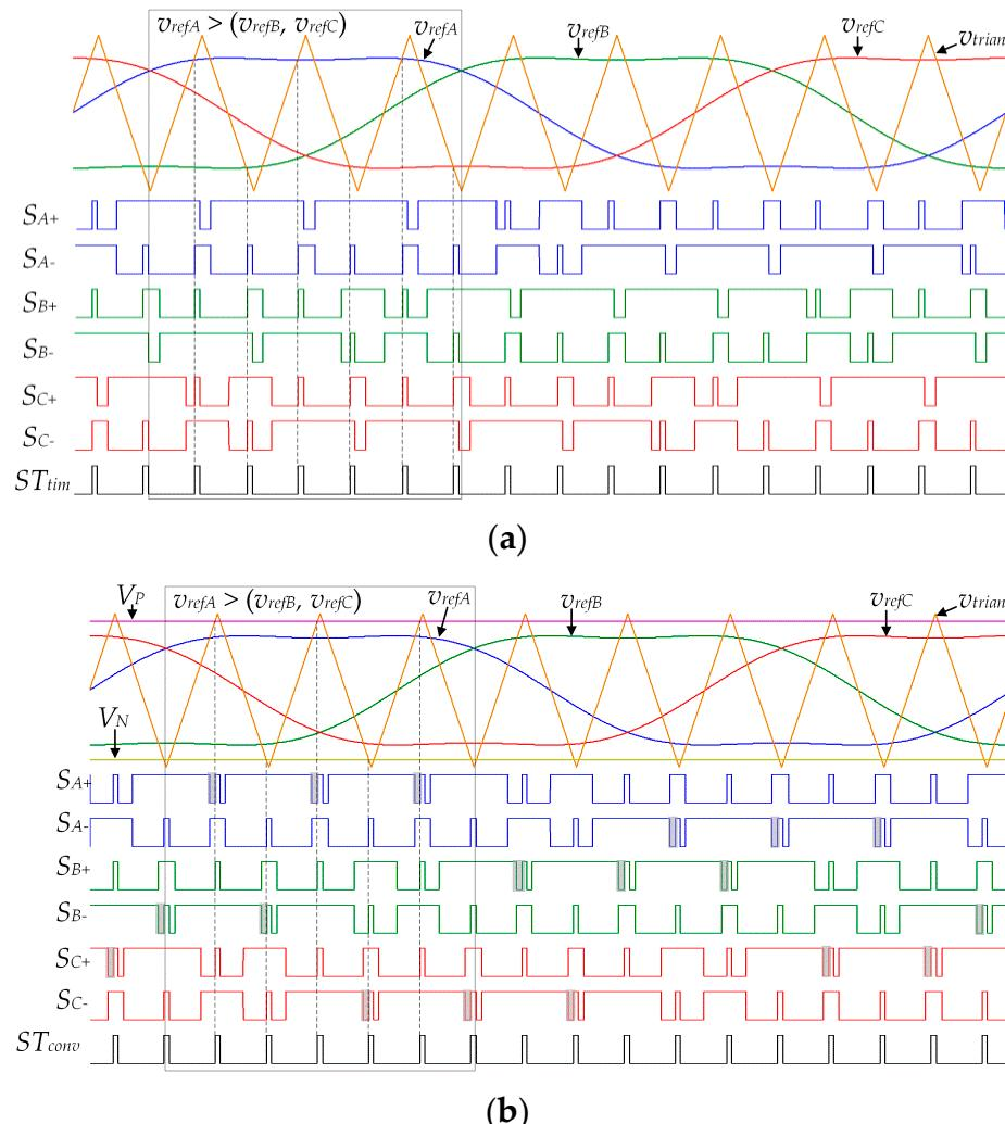
**Figure 2.** Waveforms of the zero-sync STS injection method (a) and the conventional STS injection method (b), with  $0 < D_0 < D_{0,max}$ .
