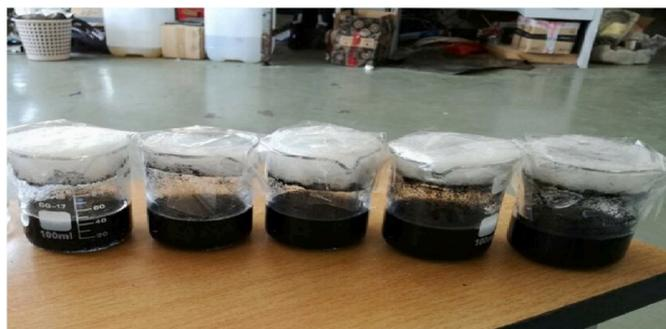
Fig. 17. Multi-walled carbon nanotubes (MWCNT) nanofluids, [52].
