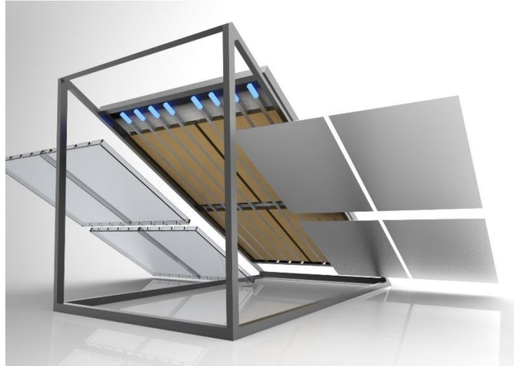
Figure 7.2. PVT-PCM collector with multi-block cooling [118].
