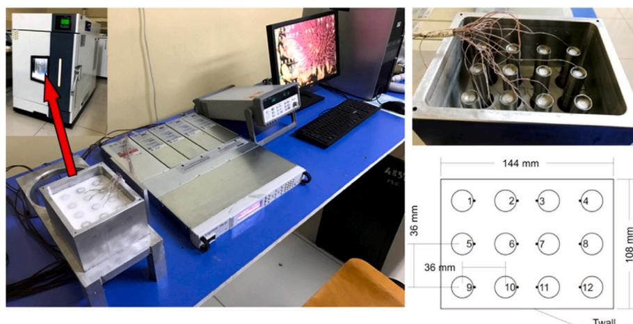
Fig. 12. Experimental layout of the simulated battery pack, [43].
