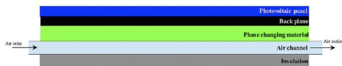
Fig. 6. Schematic of PVT air-based cooled solar panel [34].
