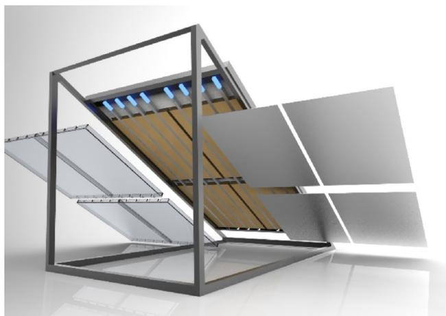
Fig. 3. PVT-PCM collector concept with four separate containers.
