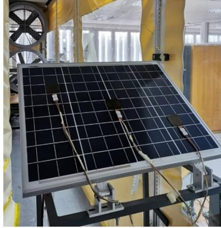
Figure 8.1. Experimental test rig layout in wind tunnel [117].
