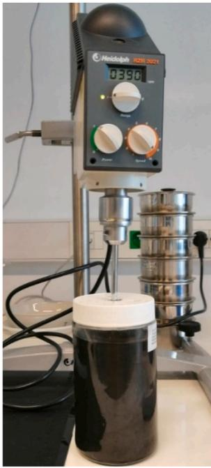
Fig. 5. Mechanical stirring of NEPCM.
