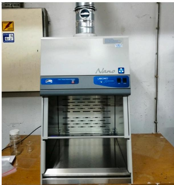
Fig. 1. LABCONCO XPert Nano Enclosure powder weighing station.
